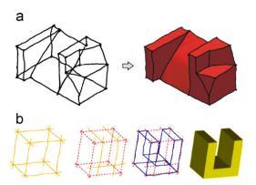
**Fig. 13.** Engineering design systems exploit domain-specific knowledge to reconstruct quite complex sketches: (a) a batch reconstruction system (reproduced from [11]); (b) an interactive system (adapted from [48]).
