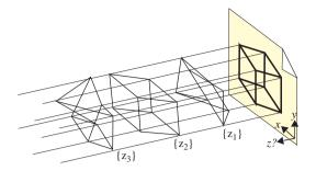
Fig. 3. Ambiguous interpretation of a 2D sketch in 3D: there are infinitely many objects that project to the same 2D input. Reproduced with permission from [11].
