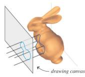
**Fig. 7.** Sketches are embedded into 3D by projecting onto a drawing canvas, or perhaps onto existing geometry.
