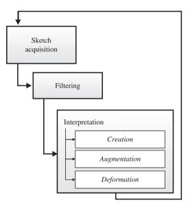
**Fig. 2.** The SBIM pipeline: after acquiring and filtering the input sketch, the sketch can be interpreted as an operation in 3D.
