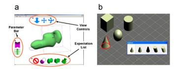
**Fig. 21.** Suggestive interfaces use expectation lists to disambiguate input: (a) interface of ShapeShop [16], showing an expectation list for operations. (b) Interface of GIDeS [45], showing expectation lists with different shapes for user confirmation.
