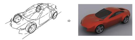
Fig. 1. Creating a 3D model from a sketch requires complex software and an expert user to understand what the sketch depicts and translate that to 3D. SBIM attempts to simplify or automate the process.
