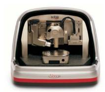
mension Edge AFM system features a drift-compensated stage that permits collection of the finer details critical to proper material identification, protects fragile tips and samples, and diminishes tip artifacts. *Veeco Metrology Inc*, 112 Robin Hill Road, Santa Barbara, CA 93117, http://www.veeco.com
