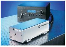
The laser's automated harmonic crystal shifter maintains constant output power for more than 20 000 hours and helps reduce maintenance costs. Its PosiLock beam position sensor and feedback loop result in very high beam position stability over the life of the laser. The AVIA 355-5 has been designed for easy integration with a laser head measuring only 491 × 216 × 141 mm³. Coherent Inc, 5100 Patrick Henry Drive, Santa Clara, CA 95054, http://www.coherent.com
